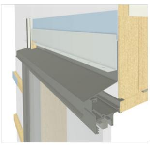
2.1 Install the Cavity Vent Strip so that the bottom of the vent strip is flush with the underside of the bottom plate (or flush with the underside of the cavity battens). Note: A minimum 15 mm drip edge to the bottom of the UltraClad® weatherboard must be maintained at all times.
