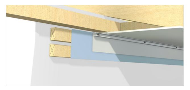
**6.1** At the top of the wall, fix the inner soffit clip through the cavity battens.
