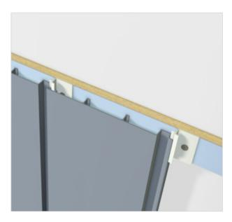
7.1 Secure the top of the weatherboard to each stud at a maximum of 600mm centres with locator clips fixed with 50mm (65mm when there is substrate) stainless screws.
