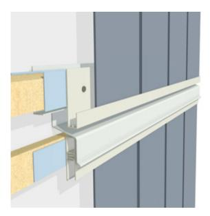
10.2 Inter-storey drainage joints are required for three storey construction, with powder coated aluminium flashing colour matched with weatherboard, as detailed and in accordance with UltraClad® requirements.
