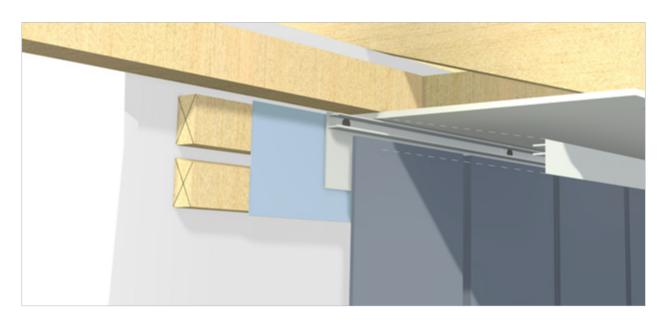
**9.2** Measure and cut the outer soffit clip to finish tight between the internal and external corner flashings and secure in place.
