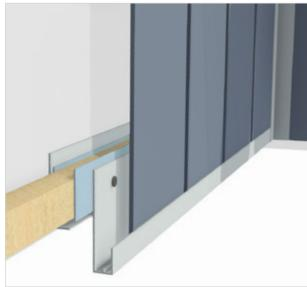
7.2 Install boards from the starter strip, working upwards, ensuring they are true to line and level. Keep cladding lines consistent and true along walls and around corners.
